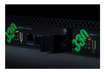
grade longevity in mind with MTBF figures in excess of 15 years and a power consumption of less than 35 Watts per blade as key design criteria. Two VB330 blades can be fitted in one 1RU chassis. The embedded VB330 solution presents the ideal option for applications in networks where concerns over energy drawn and rack space might constitute a concern.
